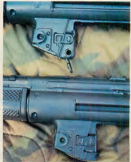
To further frustrate illegal auto-converters, H&K makes different magazine wells for auto and semiauto models: MP5 (above) has flapper release that prevents interchange with HK94 parts.
